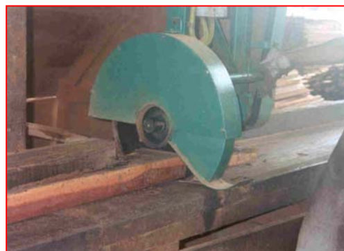
Protection of the destopadeira buzz saw
